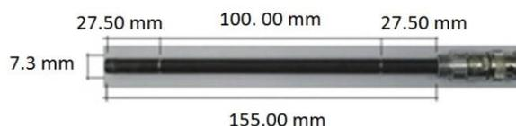
**Figure 1.** Pencil ionization chamber prototype developed at the IPEN.
