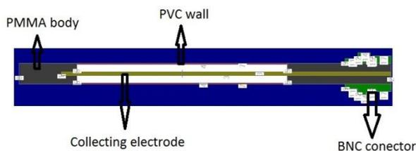
**Figure 2.** Pencil ionization chamber simulated by the MCNP-4C Monte Carlo code.
